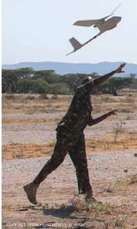
A Kenya Defence Forces Soldier launches an AeroVironment RQ-11 Raven unmanned aerial vehicle during training with the U.S. Army.
